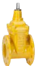
Series 06/70 Flanged gate valve Face-to-face DIN F4 DN40-600 PN10/16 Ductile iron External epoxy coating
