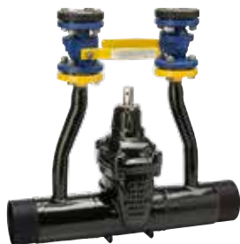
Series 46/80 Gate valve with long spigot ends and two purge points DN80-600 PN16 Cast steel GP240GH External PUR coating
